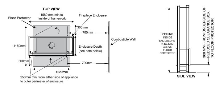
NOTE : Enclosure depth will depend on the the finished wall thickness on each side of the enclosure - see installation manual for details.
