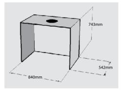
Ceiling requires 100mm airgap where flue penetrates (minimum 450mm diameter cutout).
